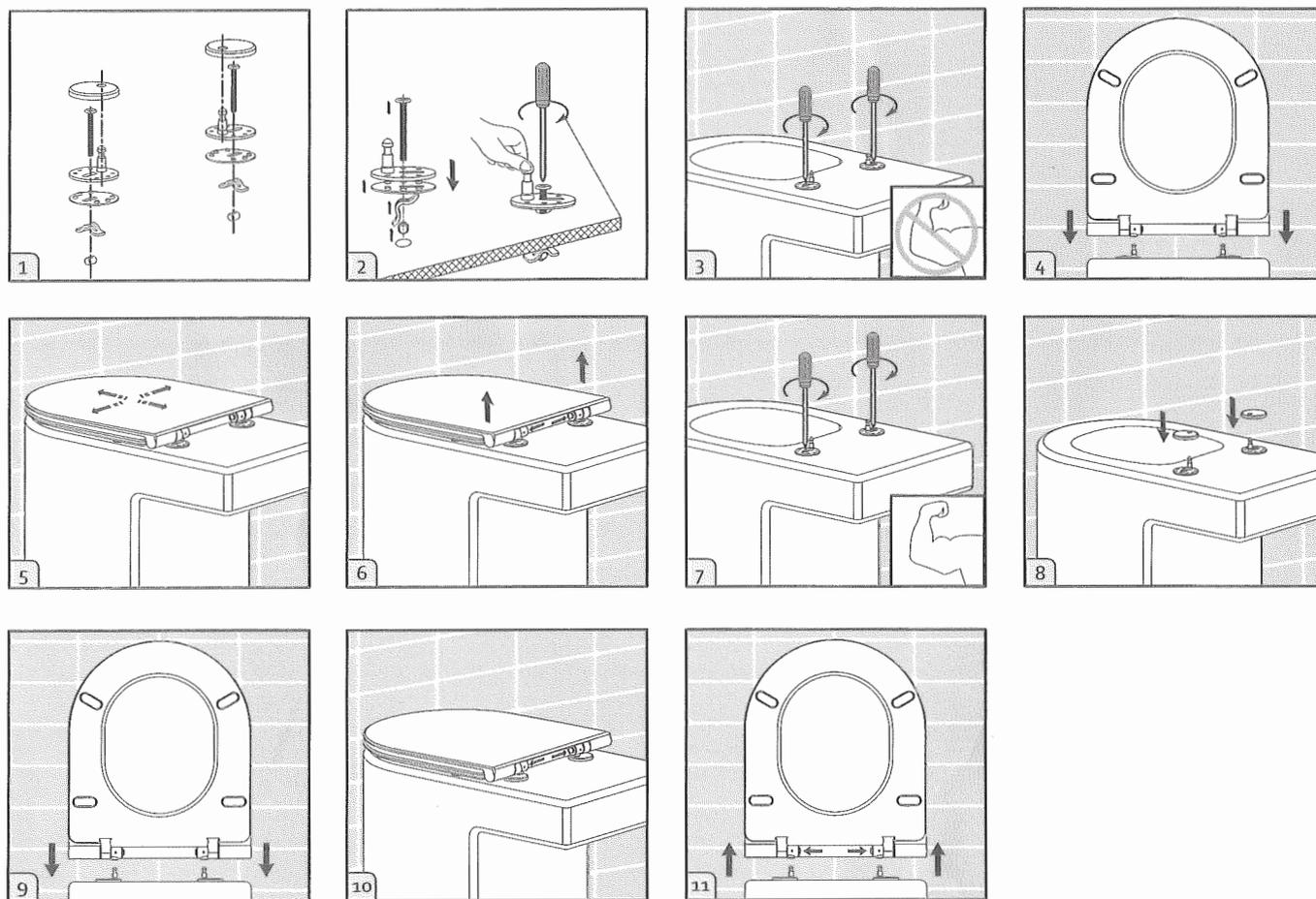
4. Before attaching the seat, move mounting bases so posts align with holes in the back of the seat. Once aligned, carefully lower the seat (holes) onto the mounting post.
